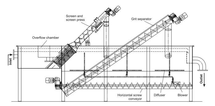
Sreening and degritting unit consists of following main parts;
